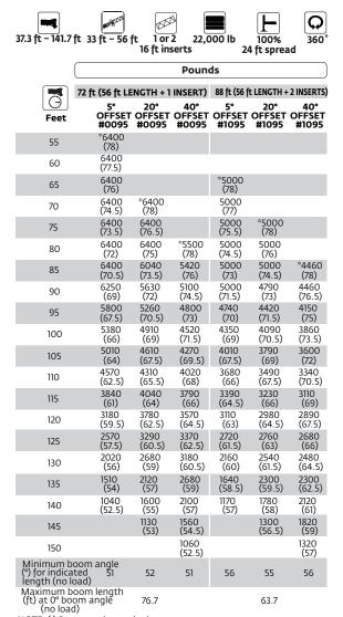
NOTE: ( ) Boom angles are in degrees. A6-829-103523 #LMI operating code. Refer to LMI manual for operating instructions. \*This capacity is based upon maximum boom angle.
